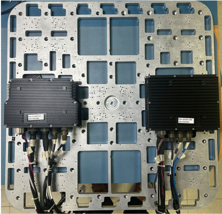
Figure 5: Top View of X and Z Axes Vibration test Setup
