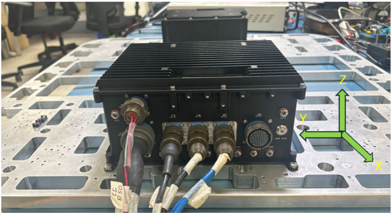
Figure 6: Side View of Y Axis Vibration test Setup
